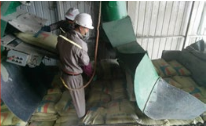
CR Cement increased its dust control efforts and deployed mobile dust collection systems in projects in Tianyang of Guangxi, Caoxi of Fujian and Jinsha of Guizhou, which effectively reduced the dust concentration in packaging and loading. The picture shows the mobile dust collection system during cement loading.
