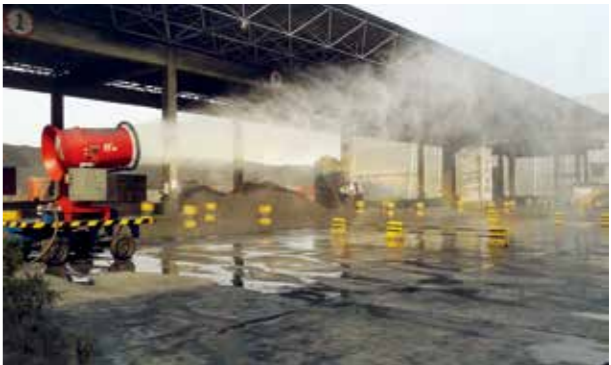
The mist sprayer in CR Power Shouyangshan Power Station
